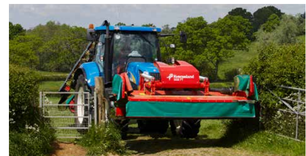
Foldable sideguards ensure narrow transport width.
